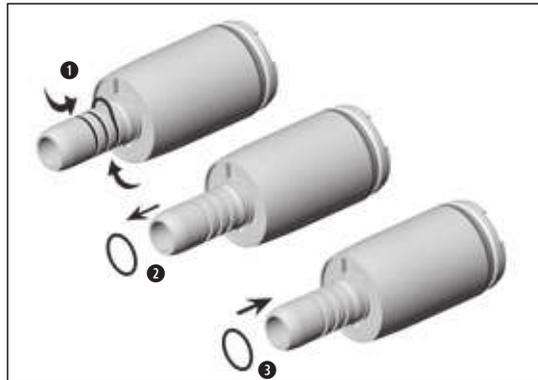
**!** Replace damaged or leaking O-rings immediately. Do not use sharp tools!
